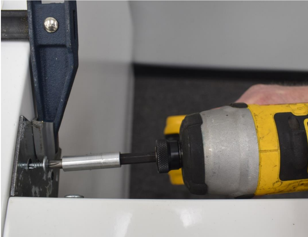
Attach Desk Bars to cabinets using self-tapping screws
