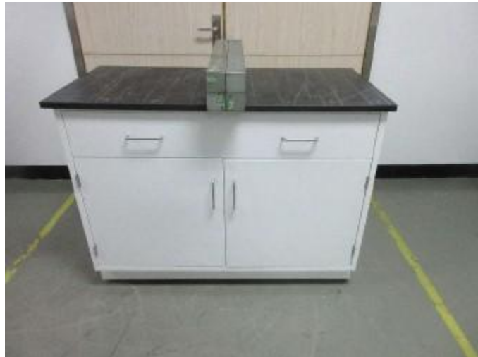
Concentrated Load Test
