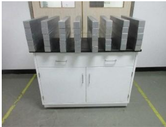
Cabinet Load Test
