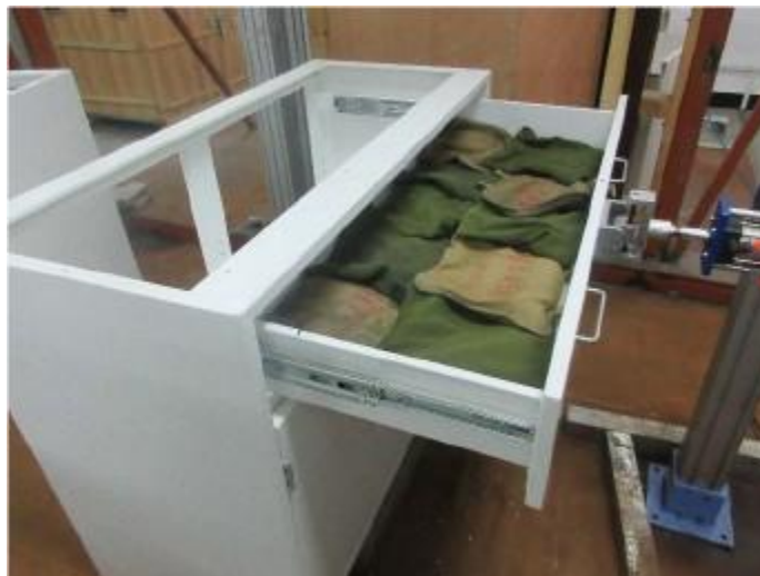
Cabinet Drawer Cycle Test
