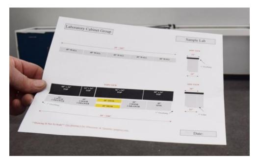
Use the provided layout drawing as a guide to position cabinets
